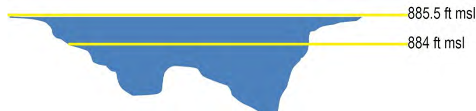
Figure 1-11. Cross Sectional Rendering of the Lowering of the Water Level at Murphey Candler Lake
