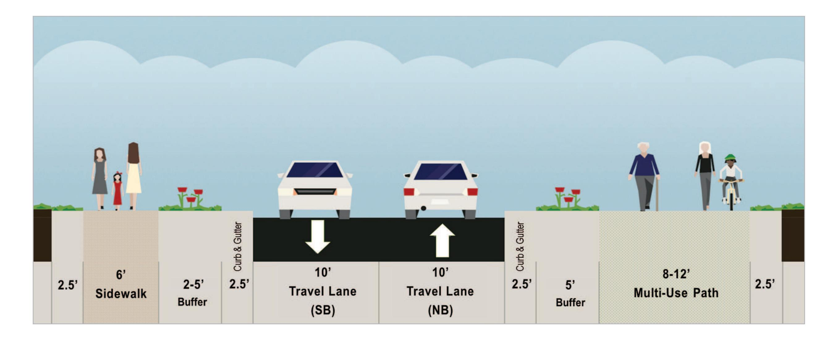
Two 10' travel lanes with 6' sidewalk on the west and 8'-12' multi-use path on the east with turn lanes as needed.
