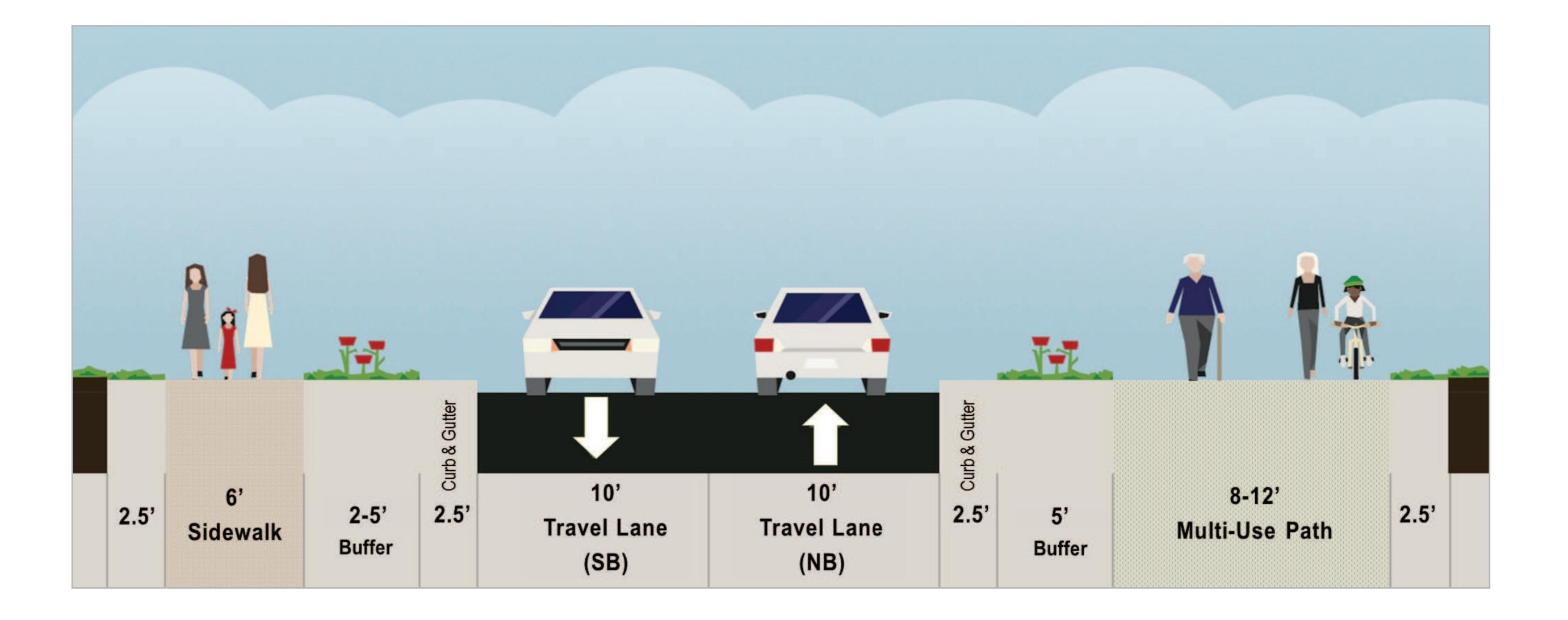
Two 10' travel lanes with 6' sidewalk on the west and 8'-12' multi-use path on the east with turn lanes as needed.
