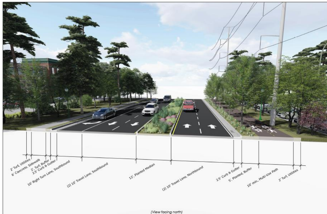
One 10' southbound right turn lane with four 10' travel lanes, a 12' planted median, 6' sidewalk on the west, and min. 10' multi-use path on the east. Turn lanes as needed (left turn lanes may be cut out of median).
