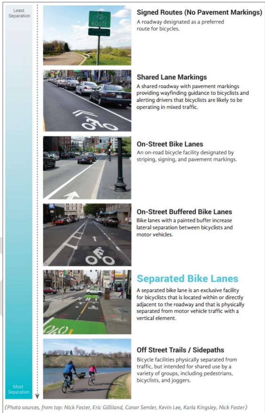
FIGURE 24. EXAMPLES OF BICYCLE FACILITIES (SOURCE: FHWA-HEP-15-025)
