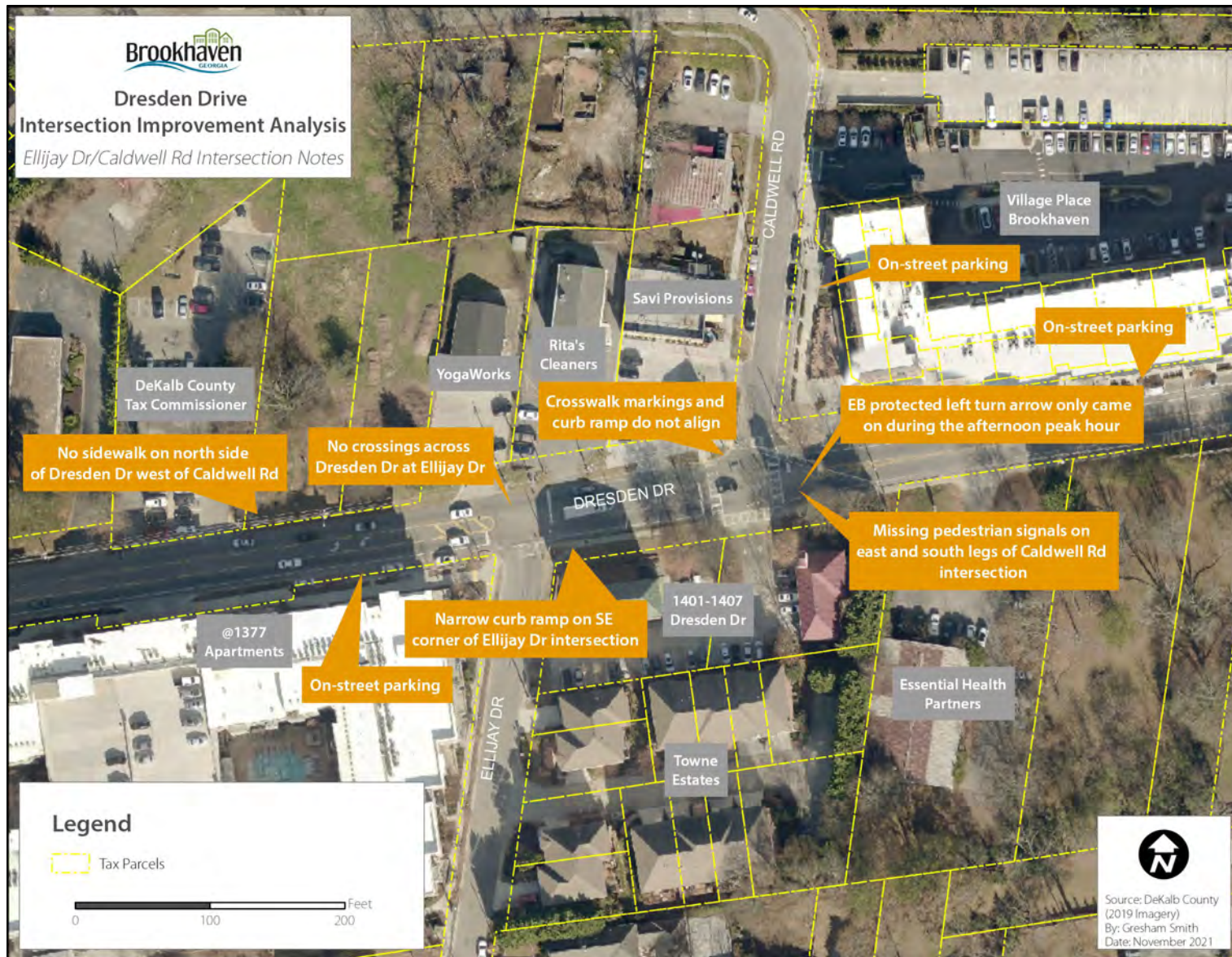
FIGURE 5: ELLIJAY DRIVE/CALDWELL ROAD INTERSECTION NOTES AND OBSERVATIONS
