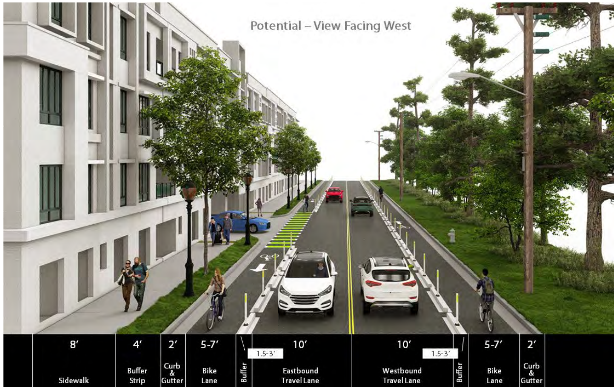
FIGURE 33: POTENTIAL TYPICAL SECTION WITH PROTECTED BICYCLE LANES
