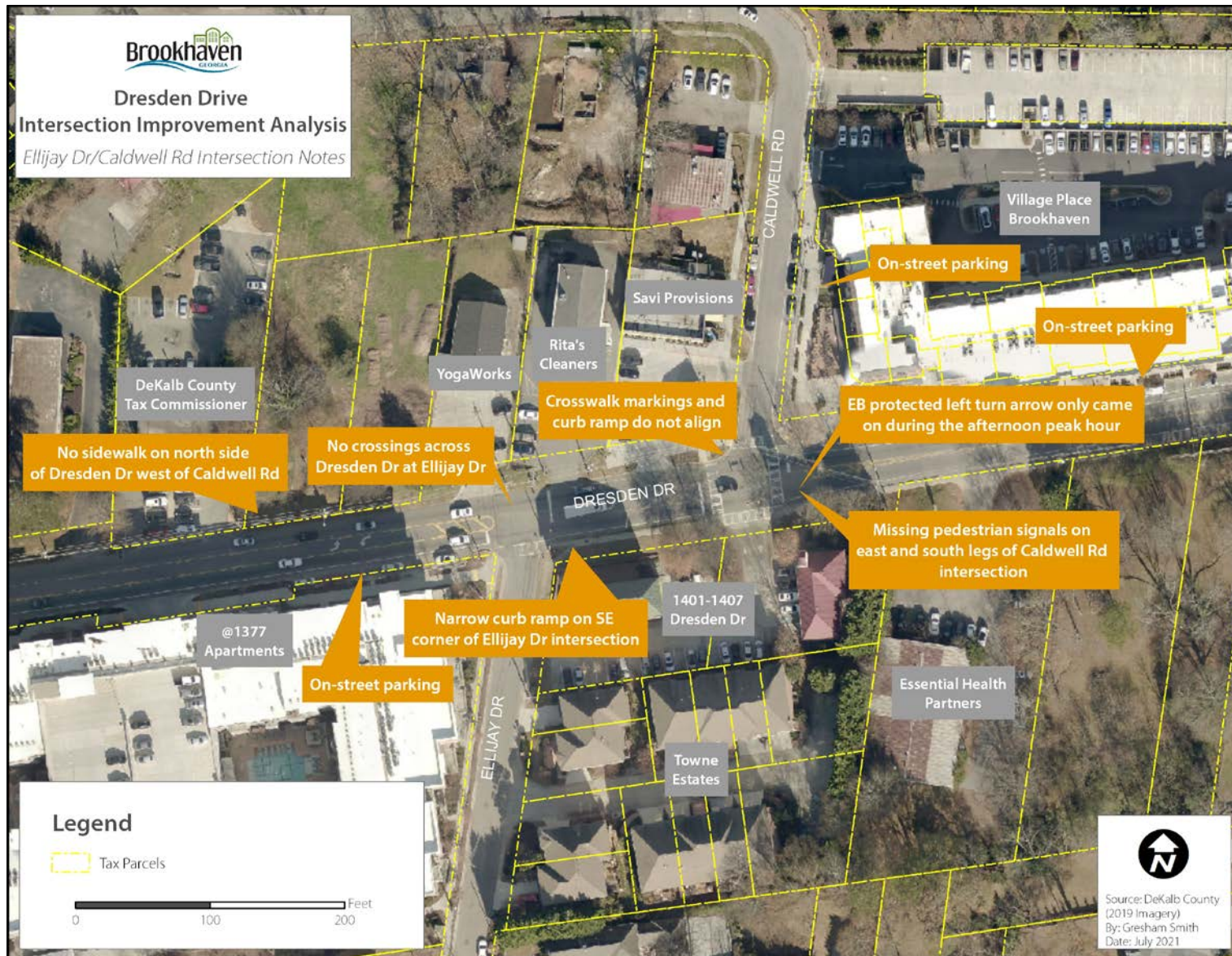
FIGURE 15: ELLIJAY DRIVE/CALDWELL ROAD INTERSECTION NOTES AND OBSERVATIONS
