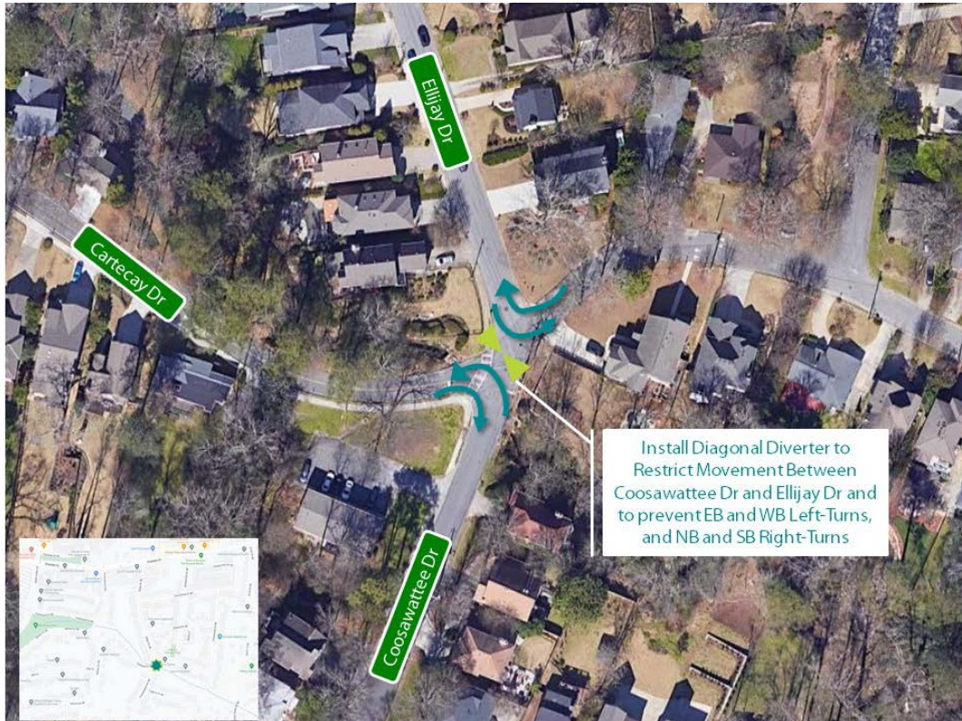
FIGURE 30: PROPOSED DIAGONAL DIVERTER AT ELLIJAY DR/COOSAWATTEE AND CARTECAY DR SOUTH OF DRESDEN DRIVE
