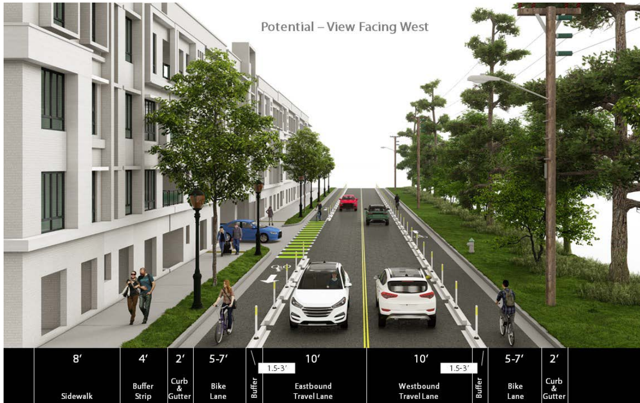
FIGURE 33: POTENTIAL TYPICAL SECTION WITH PROTECTED BICYCLE LANES
