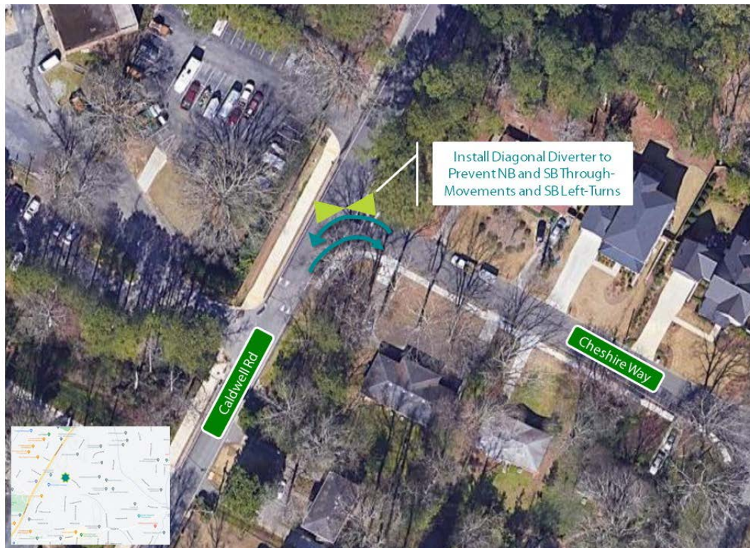
FIGURE 27: ALTERNATIVE A PART 2 - DIAGONAL DIVERTER AT CALDWELL RD AND CHESHIRE WAY
