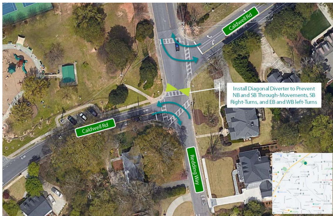
FIGURE 29: ALTERNATIVE B - DIAGONAL DIVERTER AT REDDING RD AND CALDWELL RD
