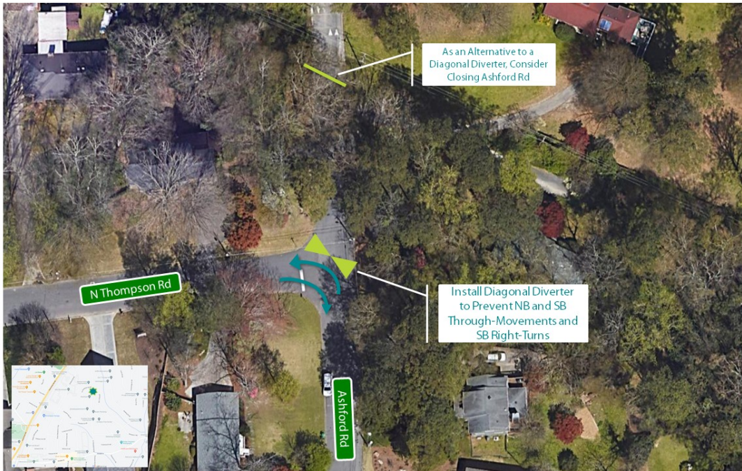
FIGURE 26: ALTERNATIVE A PART 1 - DIAGONAL DIVERTER AT ASHFORD RD AND N THOMPSON RD
