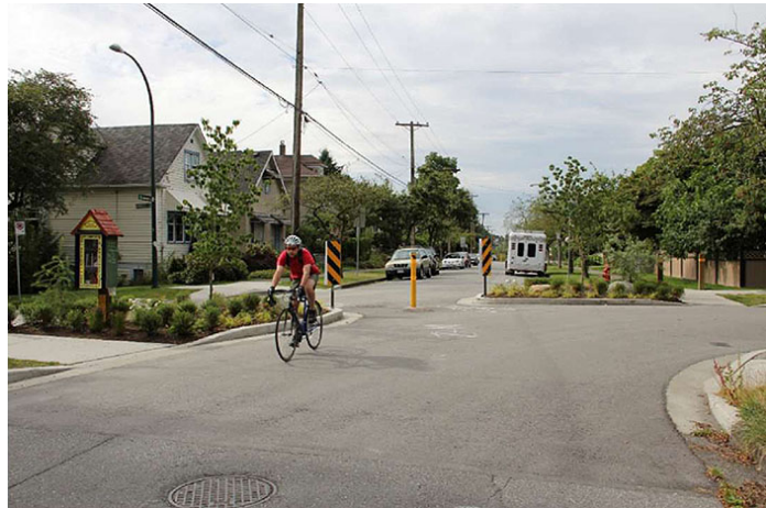
FIGURE 23: EXAMPLE OF A DIAGONAL DIVERTER
