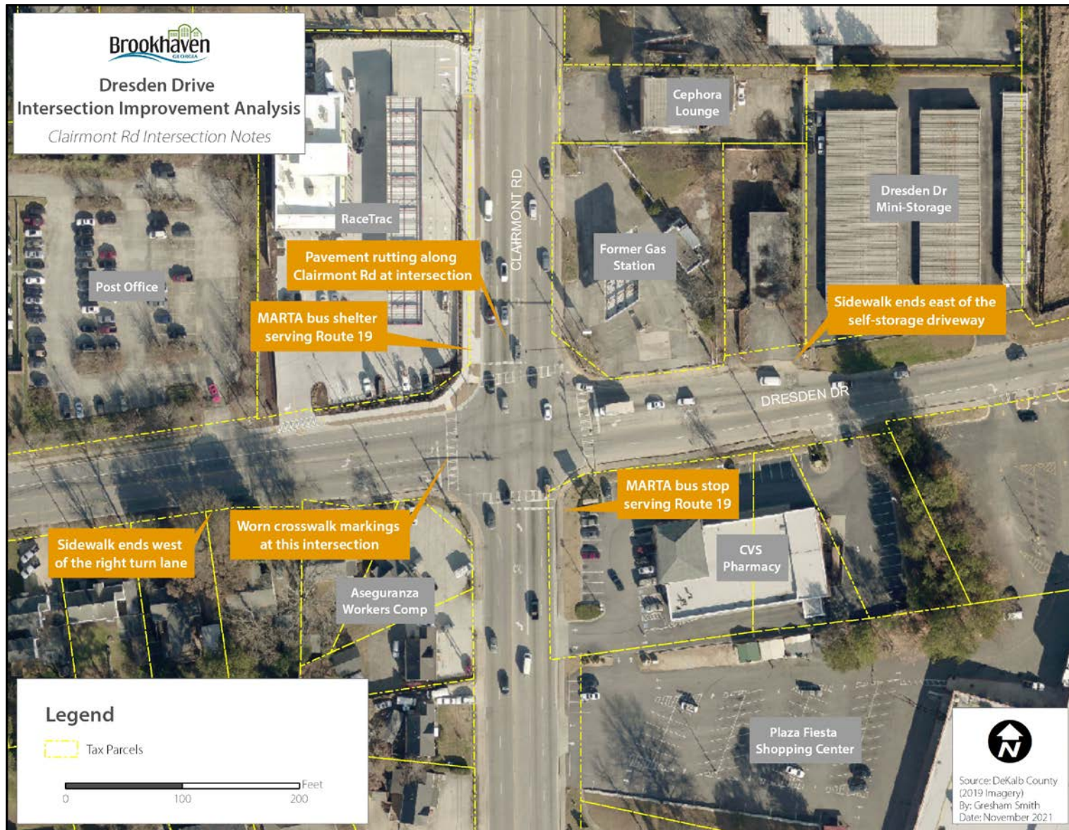
FIGURE 6: CLAIRMONT ROAD INTERSECTION NOTES AND OBSERVATIONS
