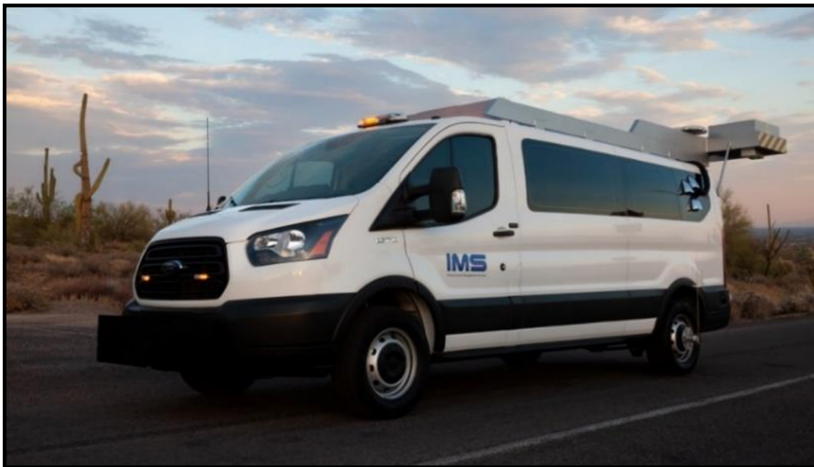
Figure 1 - IMS Road Surface Tester (RST)
