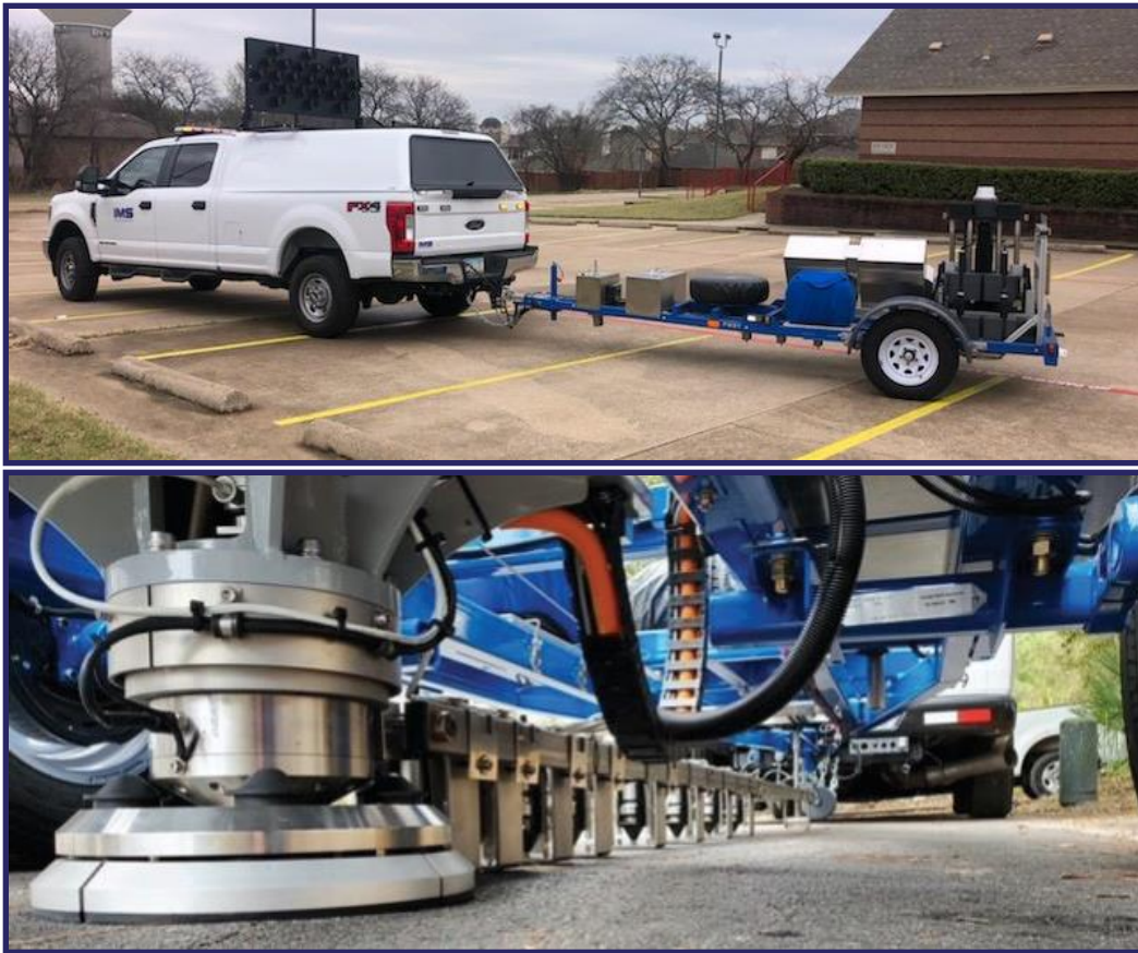
Figure 10 - Fast Falling Weight Deflectometer
