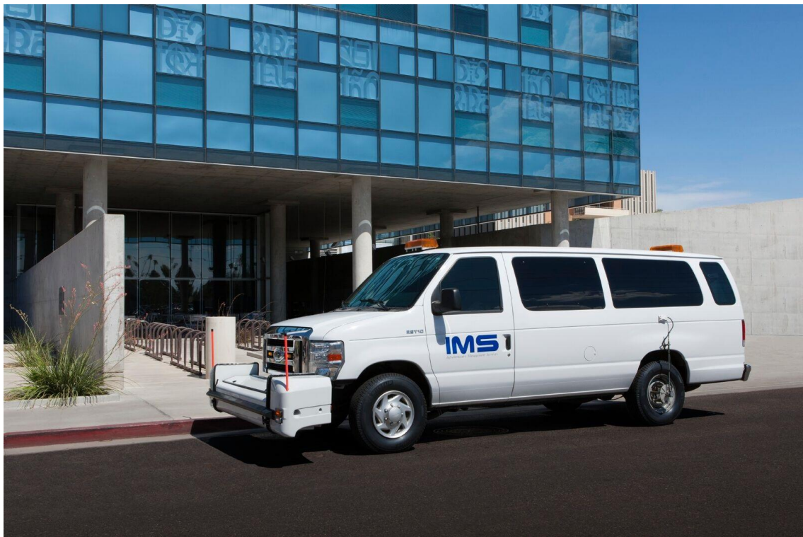
Figure 5 – Laser Road Surface Tester (Laser RST)
