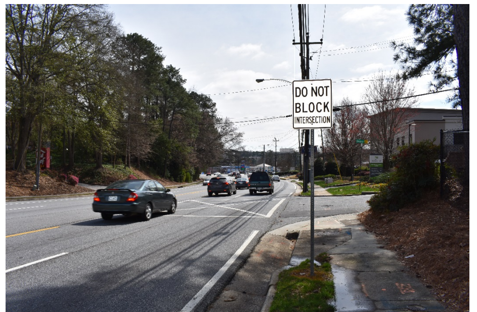
Example of Do Not Block Intersection sign and pavement markings on southbound N. Druid Hill Rd at Saxon Place
