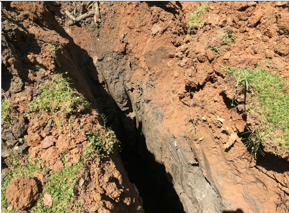
TP-3 - Approximately 2½ feet of “clean” fill cover followed by debris-laden soil and organic refuse. Groundwater encountered at 18 feet.
