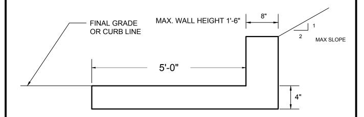
NO REINFORCEMENT REQUIRED MIN. 2500 PSI CONCRETE
