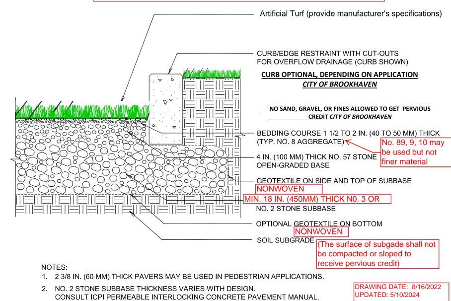
PERMEABLE SYNTHETIC TURF WITH FULL EXFILTRATION TO SOIL SUBGRADE
