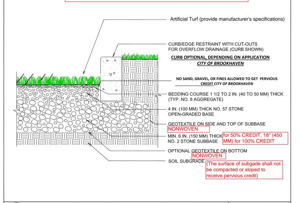
PERMEABLE SYNTHETIC TURF WITH FULL EXFILTRATION TO SOIL SUBGRADE DRAWING NO.
