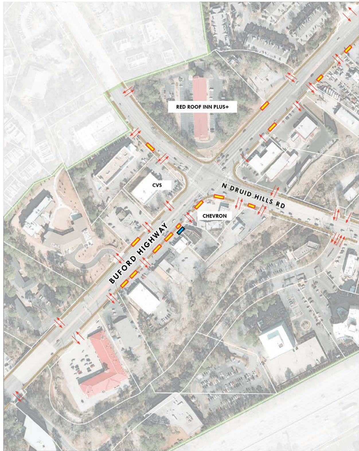
Figure 3.12 - Proposed Curb Cut Consolidation: Buford Highway at N. Druid Hills Rd.
