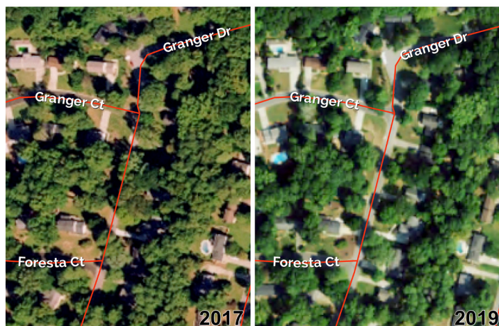
Figure 9. | A comparison of NAIP imagery in 2017 (left) and 2019 (right). The relatively large off-nadir angle in 2017 causes trees to lean in one direction and appear to cover a larger area than they actually do. This can cause overestimation in the canopy cover data.
