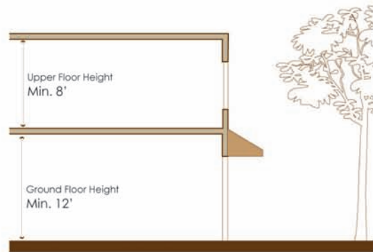
Example: Building cross section / floor height
