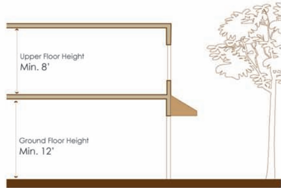
Example: Building cross section / floor height
