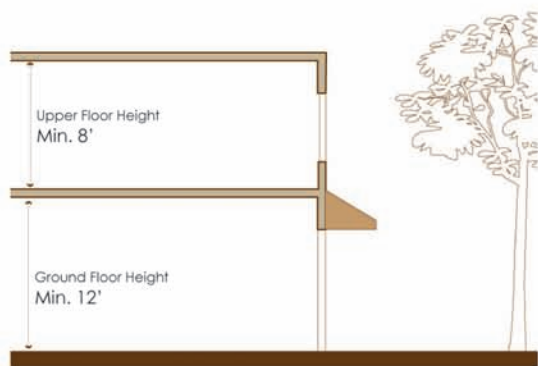
Example: Building cross section / floor height
